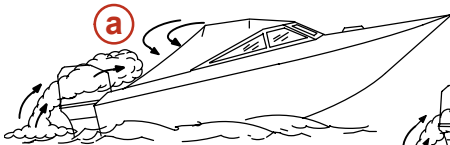
a - Running the boat with the trim angle of the bow too high.
