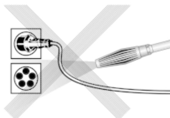
**Never direct the water jet at a power socket !**
