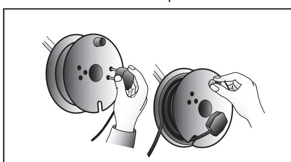
To recoil the hose: Place the steam plate end of the hose into the side aperture of the spool and then wind the hose onto the spool.
