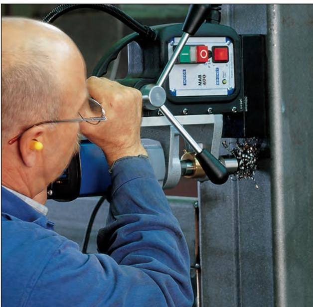
**Horizontal drilling: No problem.** The stable, steady position for precise working results is created by high electro-magnetic power. Lubrication is now made with the high-performance lubrication spray by BDS: See page 54.
