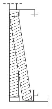
REPLACING THE FILTER Slide the filter gently upwards and prise it over the lip.
