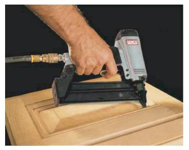
**Sequential Actuation Trigger** (also known as restrictive trigger or trigger fire) operates in the following a sequence - depress the safety element at the nose of tool against the work surface then pull the trigger. After each fastener is driven, release the trigger and lift the tool off the work surface before starting the sequence again. This trigger is recommended and acceptable for most applications.
