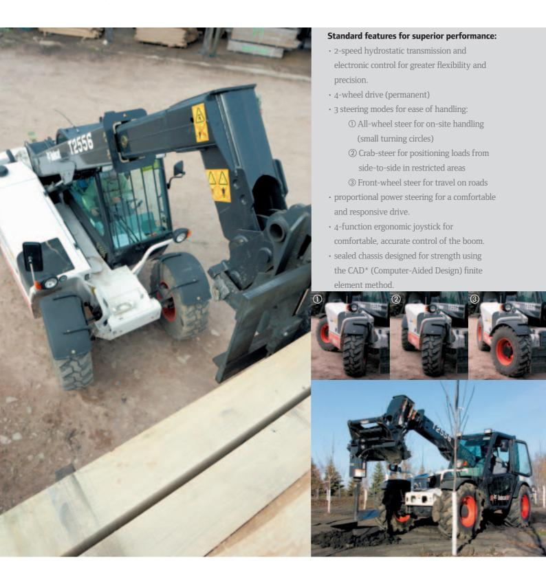
These features are all standard on Bobcat® telescopic handlers to ensure superior performance. Bobcat® telescopic handlers are assembled using state-of-the-art components utilising the latest intechnological developments.
