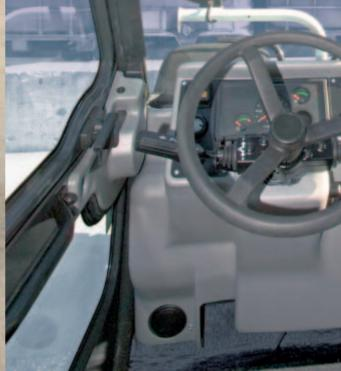
Two outer rear-view mirrors are fitted as standard, throughout the range. The cabin Bobcat® telescopic handlers rests on 3"Silentbloc" shock absorbers and is fitted to the chassis via the patented "Zebullon" suspension system, which absorbs impact energy when operating the telescopic handler.
