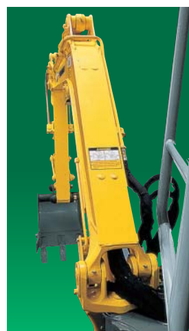
To prevent damage to the hydraulic hoses, they are housed in the inner boom for safety.
