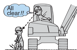
The audible traveling alarm signals people nearby when the machine is being moved.
