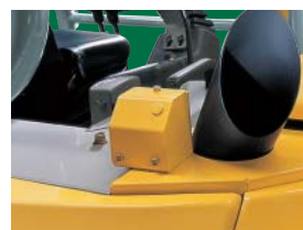
The audible traveling alarm signals people nearby when the machine is being moved.
