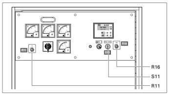
R11.... Voltage adjust potentiometer Allows to adjust the output voltage
