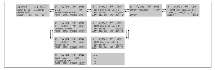
The menu flow is similar in the CONTROL SETUP, POWER SETUP and SYSTEM SETUP.
