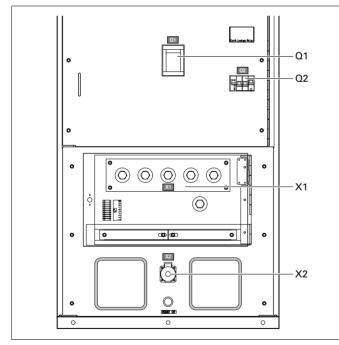
When the sockets-option is installed, circuit breaker Q1 does not only interrupt the power supply towards X1 but also towards X2.
