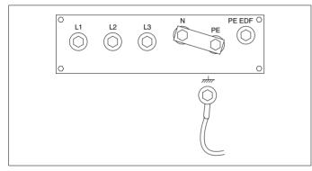
When EDF-option is installed, the unit operates as EDF-unit when the earthing, the PE and the PE EDF terminals are connected to each other (see figure below). In this case, an earth leakage at the side of the generator will switch off the circuit breaker. An earth leakage at the side of the load will not switch off the circuit breaker.
