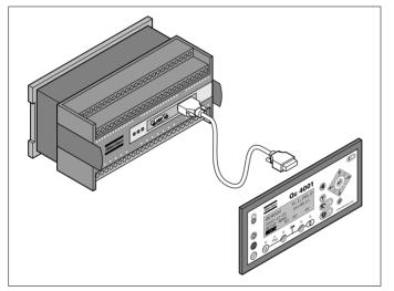
The Qc4001<sup>TM</sup> module is located inside the control panel, and communicates with a display unit, located in front of the control panel. This control module will carry out all necessary tasks to control and protect a generator, regardless of the use of the generator.
