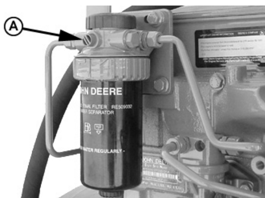
Final fuel filter bleed screw
