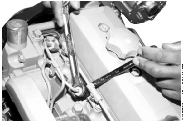
Bleed fuel system at fuel injection nozzles
