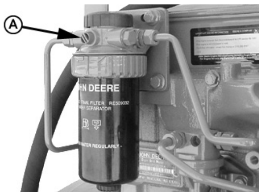
Final fuel filter bleed screw
