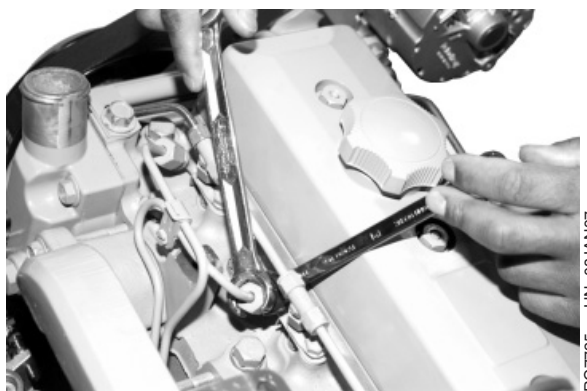
Bleed fuel system at fuel injection nozzles
