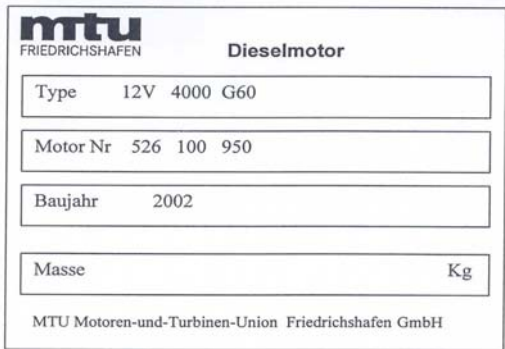
Figure 1.3: Example of generating set identification plate
